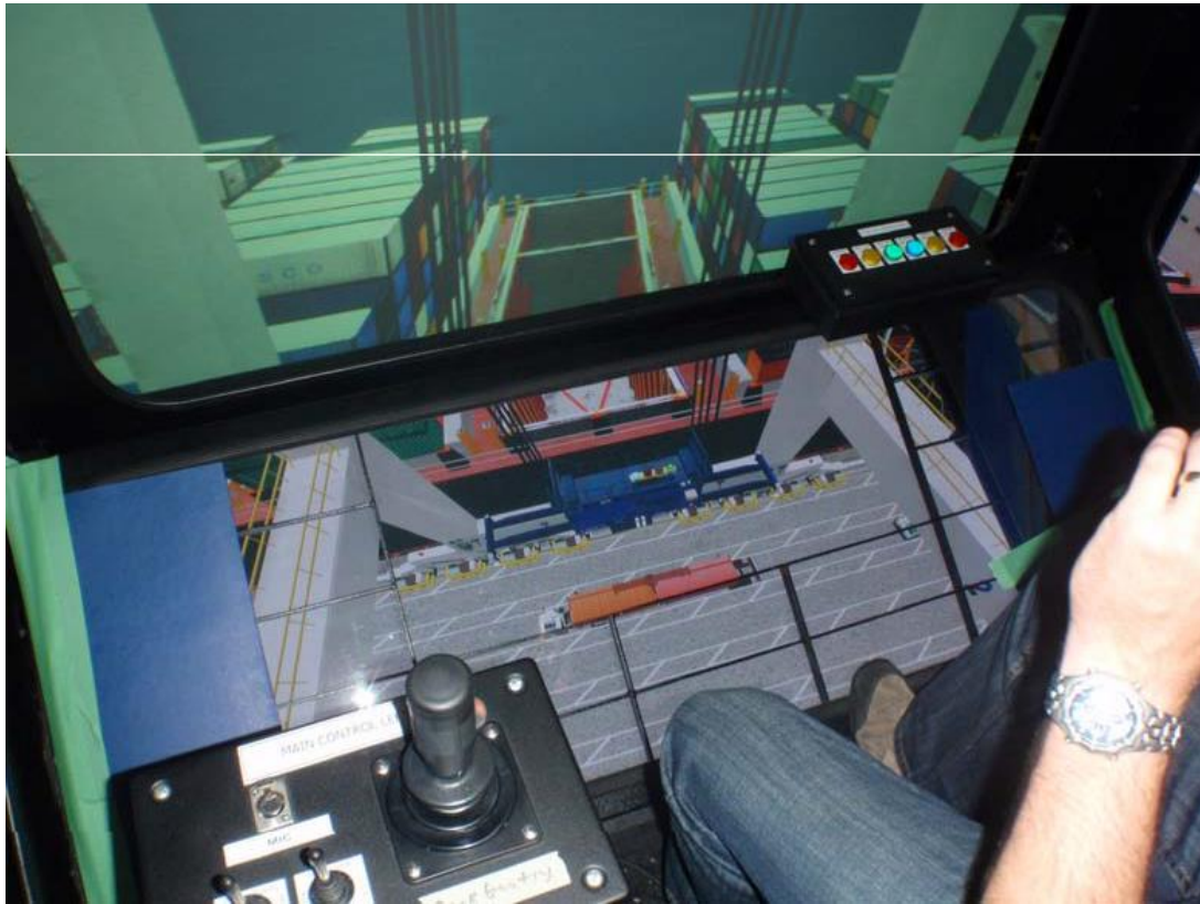
Figure 6: Antwerp portainer crane simulator
