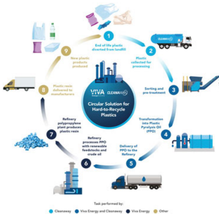
Figure 1. Cleanaway and Viva Energy proposed circular solution for hard-to-recycle plastics
