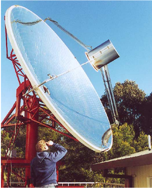
Fig. 5. 15 kW sol ammonia dissociation receiver reactor in operation on the ANU 20 m 2 dish.
