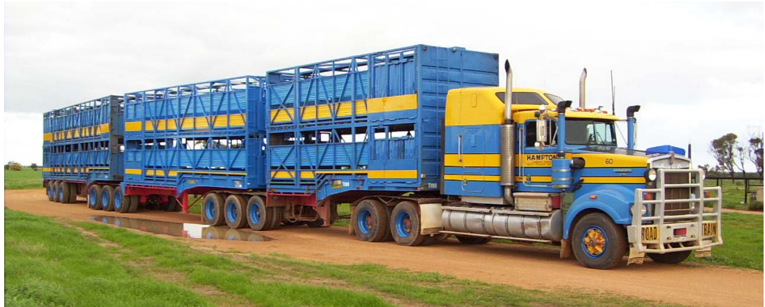
Figure 9: A B-triple 2-deck per trailer cattle transport vehicle, showing advanced engineering systems on the trailer couplings
