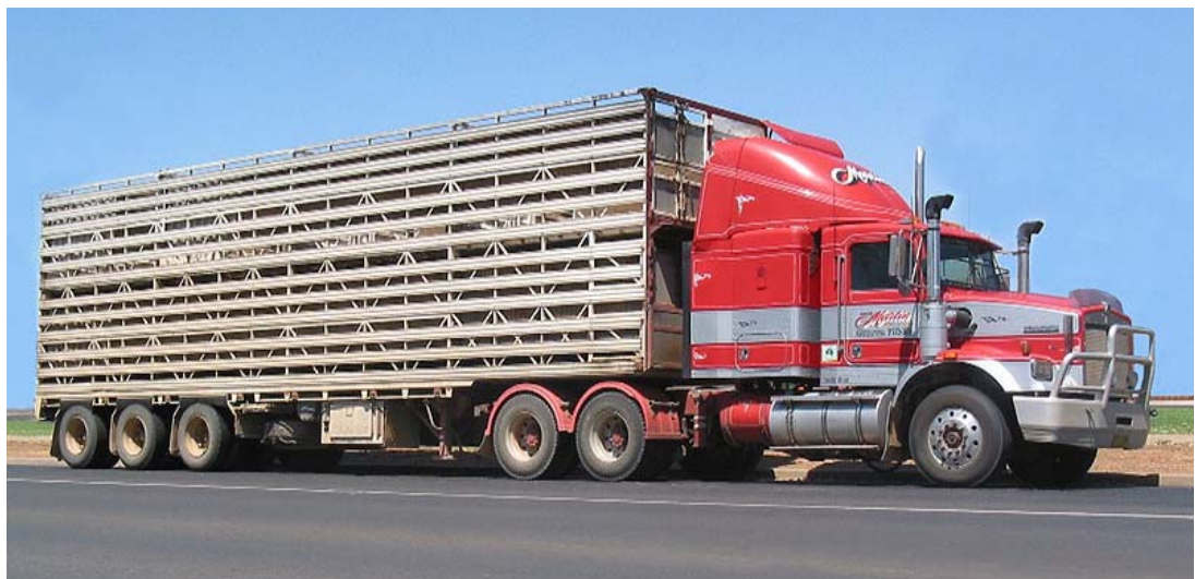
Figure 6: A standard 6-axle articulated semi-trailer configuration for livestock transport, common from the 1980s through to today
