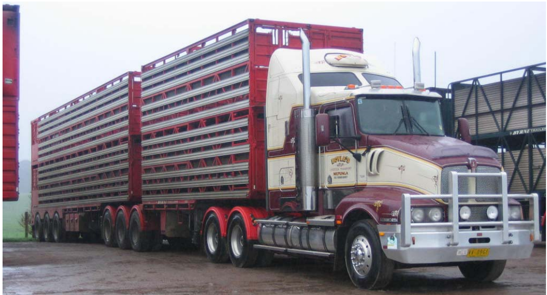
Figure 7: A B-double livestock vehicle, showing the innovative B coupling: 3 axles sitting under the beginning of the second trailer, providing much greater directional stability and responsiveness.
