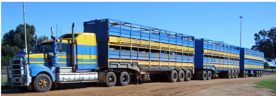
Figure 8: A standard triple road train operating in the north of Western Australia
