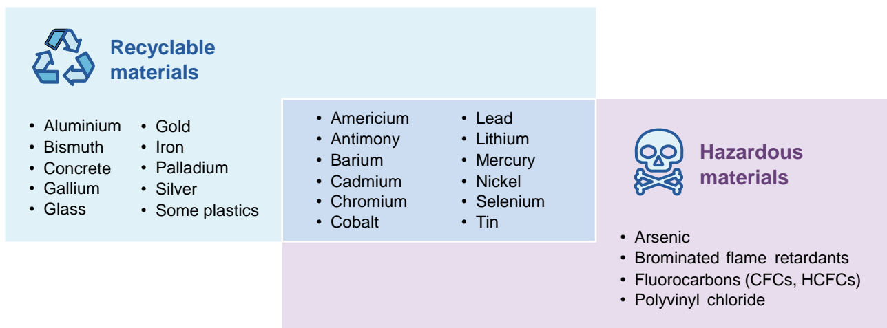
Figure 9.2 – There is a large overlap between recoverable and dangerous e-waste Examples of recyclable and hazardous e-waste materials
